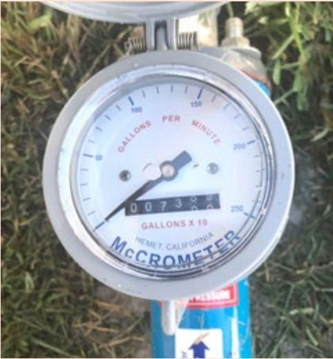
WATER PULLED FROM LAKE IS METERED- REPORT IS SENT TO SOUTH FLORIDA WATER MANAGEMENT DISTRICT EACH MONTH.
