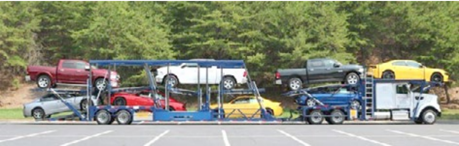
80 foot loaded car carrier weighing over 50,000 pounds
