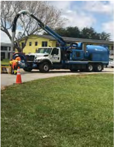
AFTER INSPECTION AND REPAIR, ALL UNDERGROUND DRAIN PIPES WERE VACUUMED OUT BY THESE TRUCKS.
