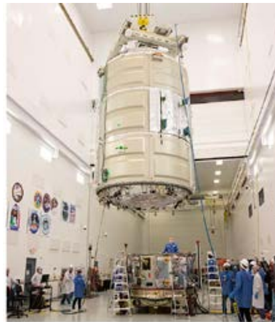
The Cygnus Service Module is mated with the Pressurized Cargo Module at the launch site
